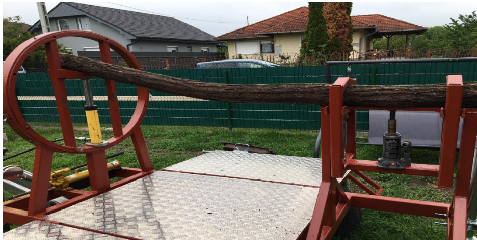
Picture 1 - Structure simulating the tension of wooden parts. Created by József Zsolt Kersák, Balatonszabadi 2023. 04. 11.11.
