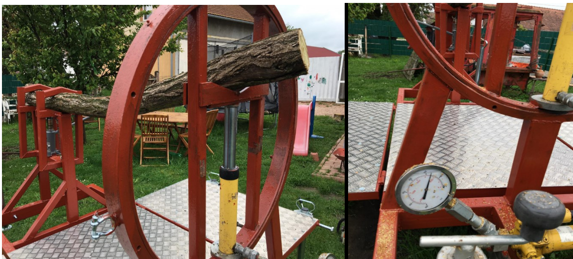
Figure 2 - Montage of a structure simulating the tension of wooden parts. Created by: Kersák József Zsolt, Balatonszabadi 2023. 04. 11.
