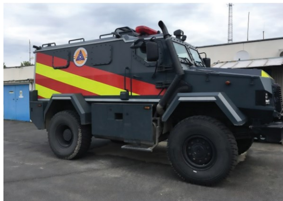
Figure 3 - Light-armoured, radiation-shielded emergency vehicle (RSV) [4]
