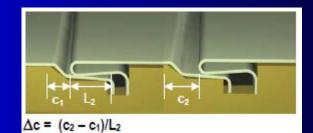
Extension are allowed only if  $\Delta c \le 0.5$ If  $\Delta f \le 0.01$  the span may be increased up to 12 m
