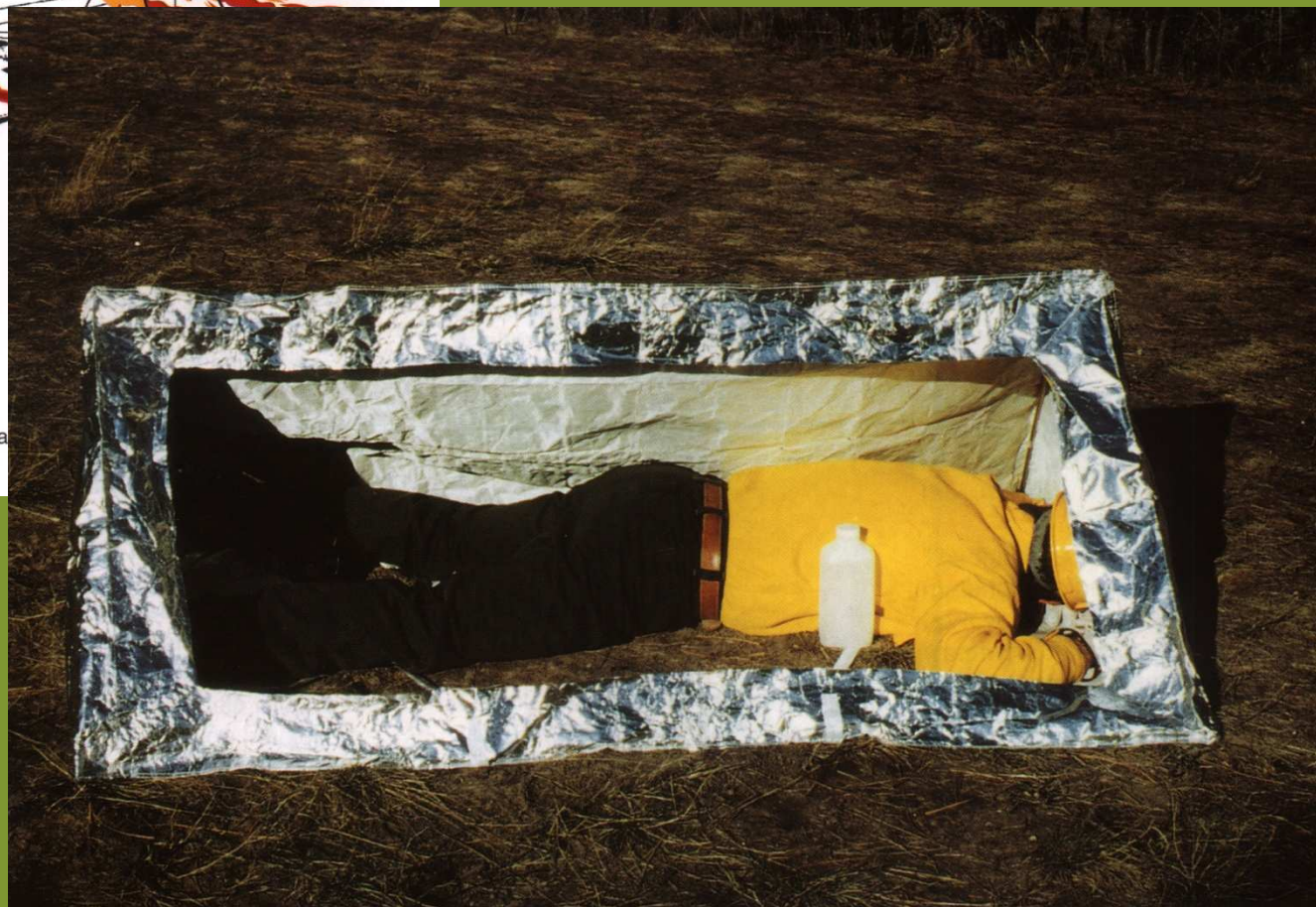
Figure 1 —The fire shelter reflects radiant heat and a
