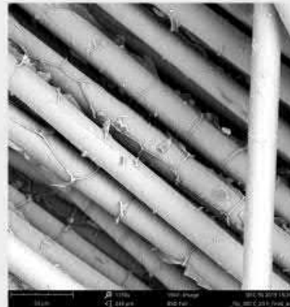
Released glass fibres after 300 °C
