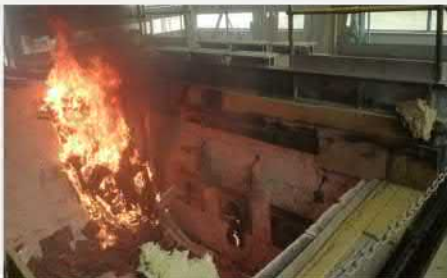
Figure 1: Fire resistance test of a light-weight roof structure (P. Tóth)
