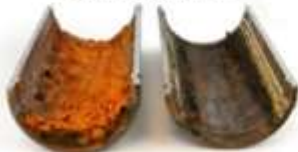
20 Month Pipe Test with Air
