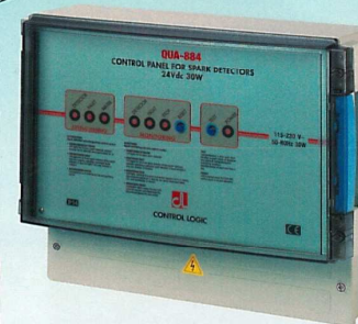
QUA-884 Control unit Used in spark detector systems with RIV-601P/S detectors. Provides visual signals of detectors alarm state and their malfunctions. Controls the extinguisher and/or the emergency stop. Executes the test sequence.
