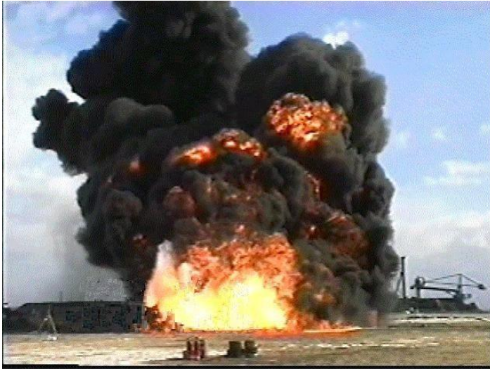
Boilover test D=5m, Arabian Crude oil, Feb. 1999
