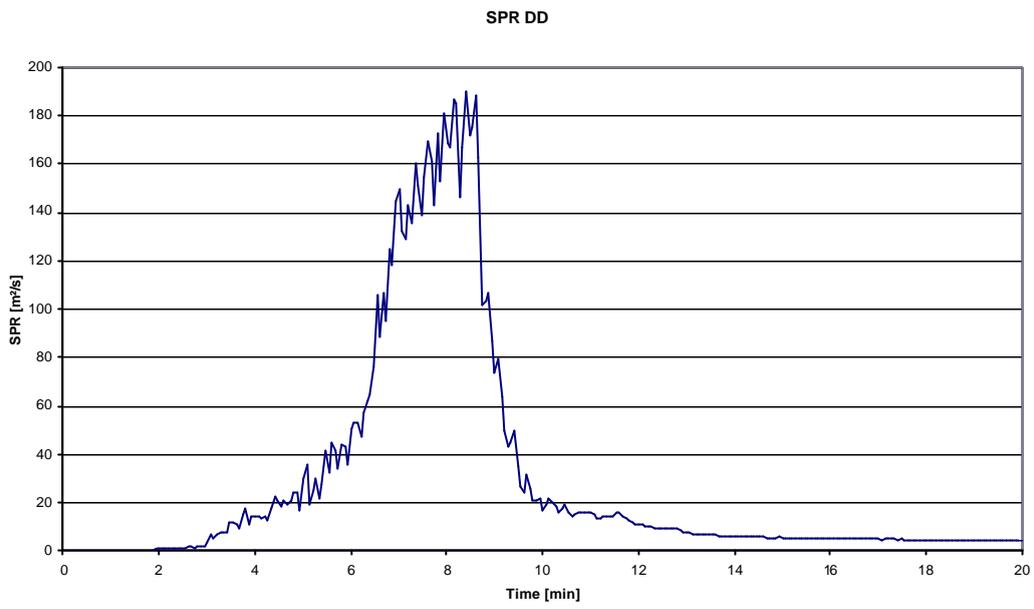
Figure B.11 Smoke production rate of product D in free standing set-up
