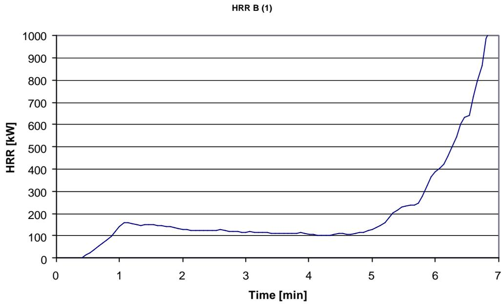
Figure A.3 Detail of heat release rate of product B in ISO 9705
