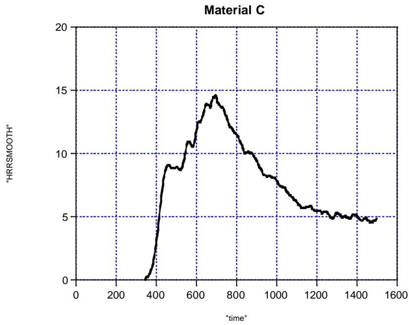
Figure C.3 Smoothed heat release rate of product C in the SBI test
