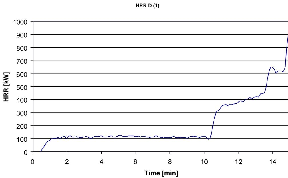
Figure A.8 Detail of heat release rate of product D in ISO 9705
