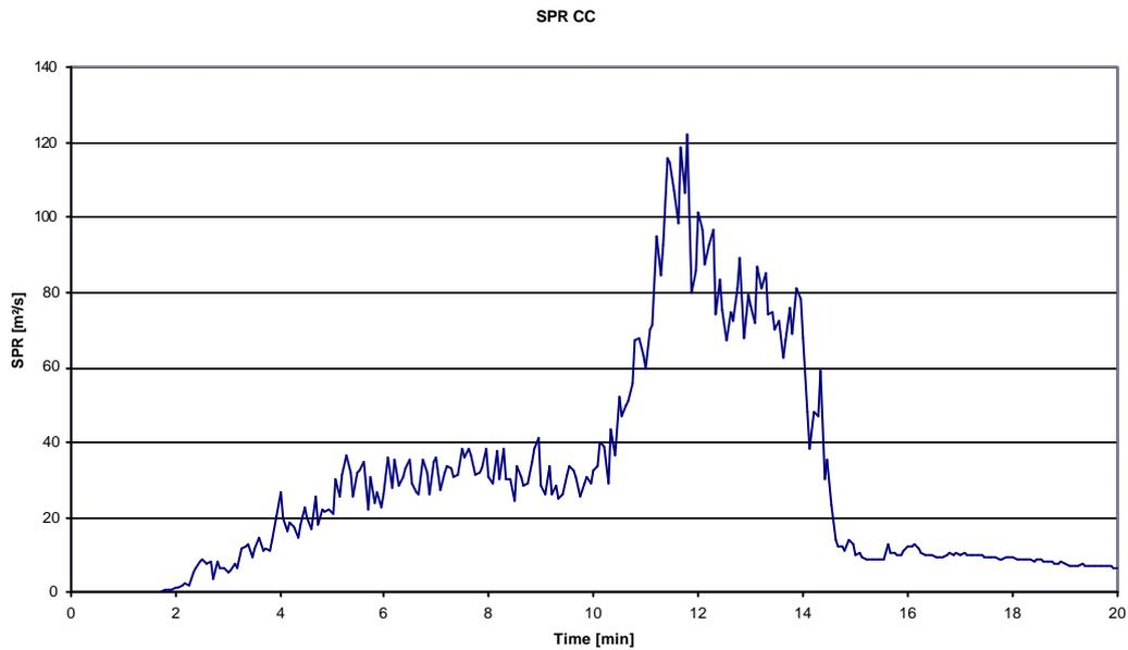
Figure B.8 Smoke production rate of product C in free standing set-up
