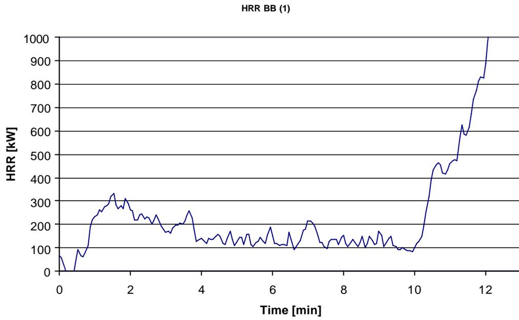
Figure B.3 Detail of heat release rate of product B in free standing set-up
