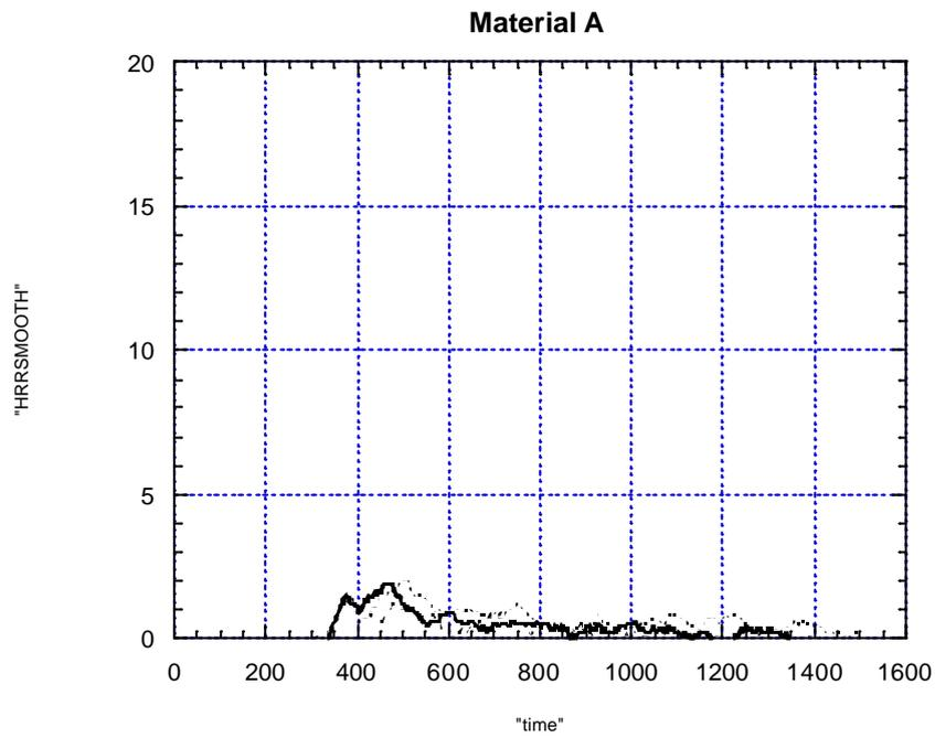
Figure C.1 Smoothed heat release rate of product A in the SBI test
