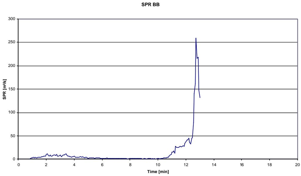
Figure B.5 Smoke production rate of product B in free standing set-up (values up to flashover)
