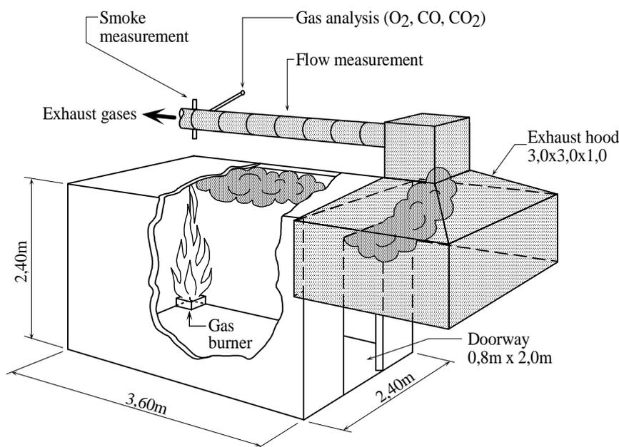
Figure 1. Schematic drawing of the room corner test set-up according to ISO 9705.
