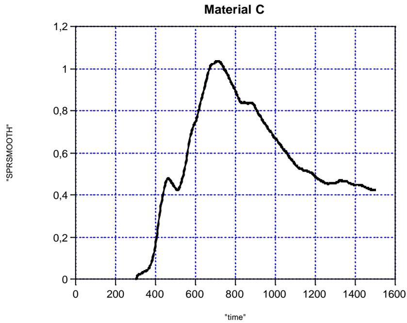
Figure C.7 Smoothed smoke release rate of product C in the SBI test
