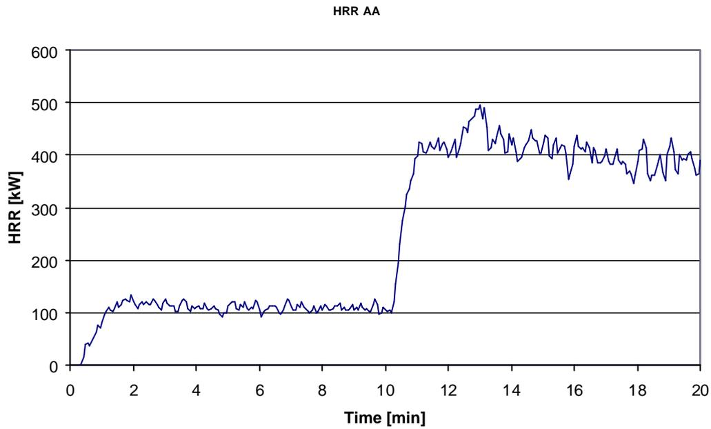
Figure B.1 Heat release of product A in free standing set-up
