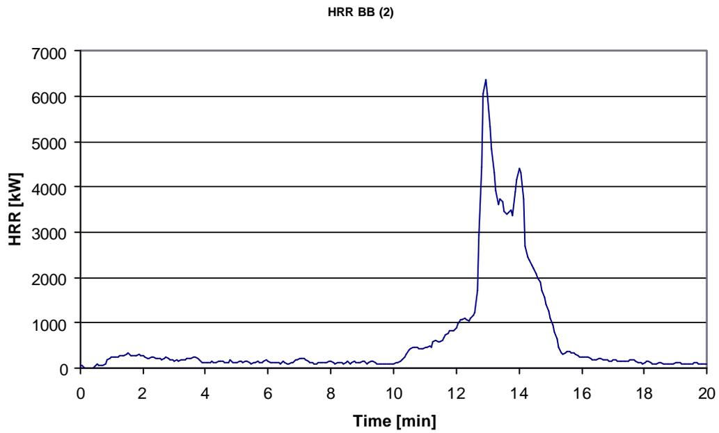
Figure B.4 Heat release rate of product B in free standing set-up
