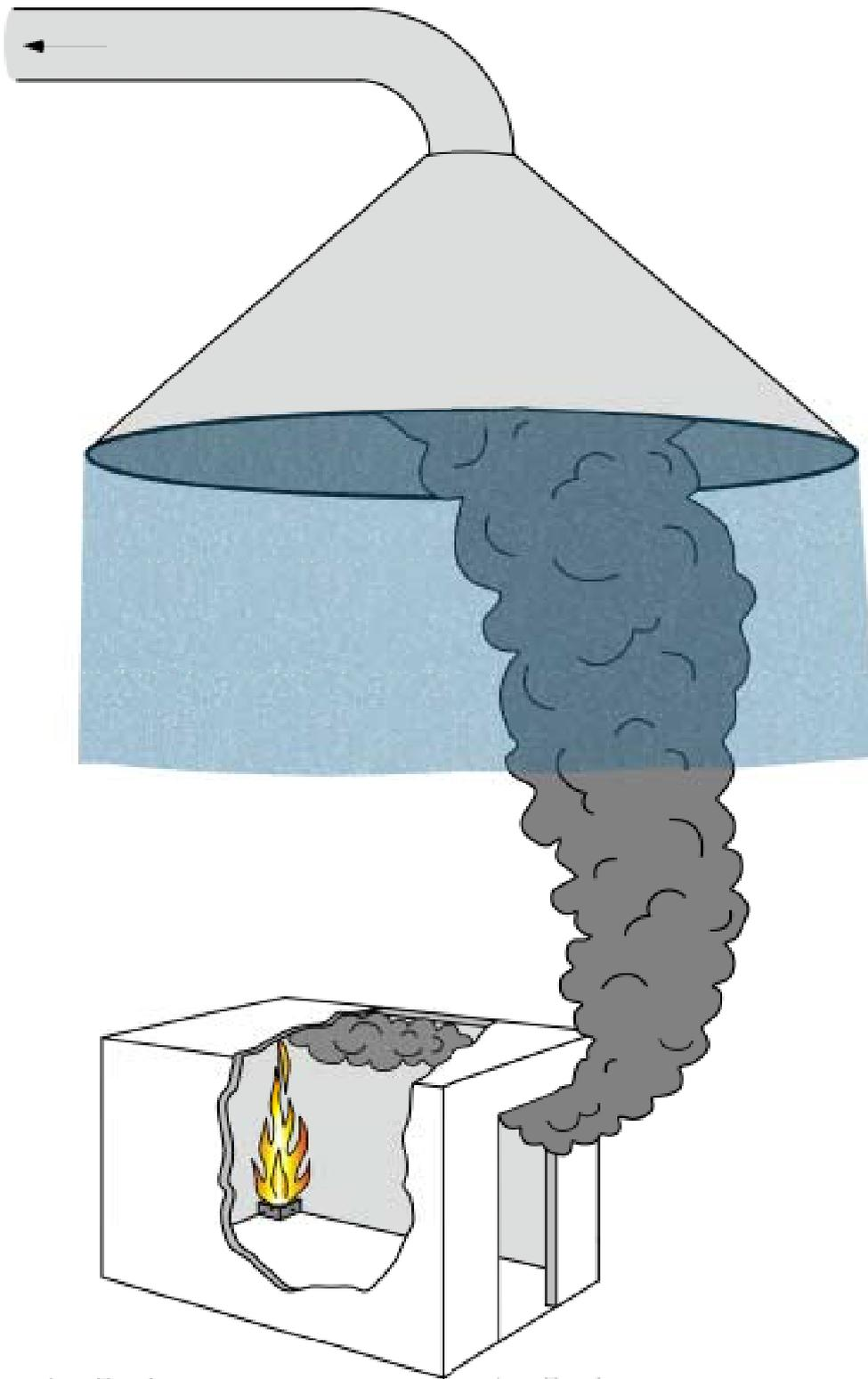
Figure 3. Schematic drawing of free-standing set-up
