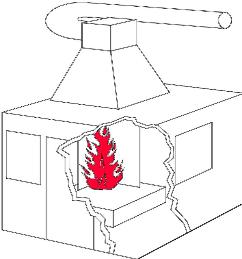
Figure 4. Schematic drawing of the SBI method.
