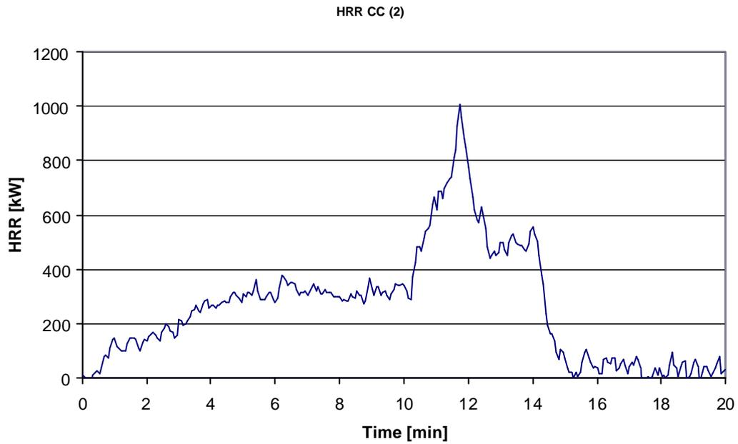
Figure B.7 Heat release rate of product C in free standing set-up
