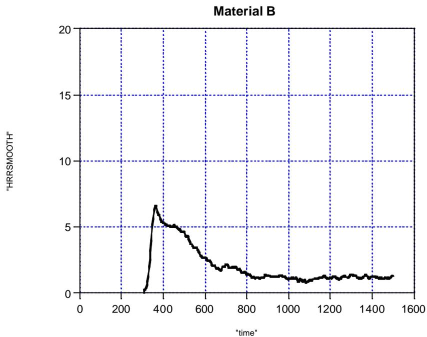
Figure C.2 Smoothed heat release rate of product B in the SBI test
