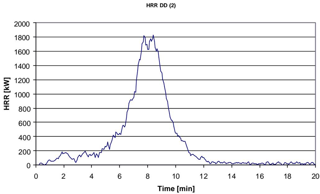
Figure B.10 Heat release rate of product D in free standing set-up
