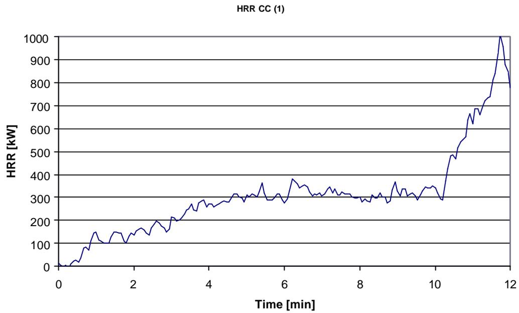
Figure B.6 Detail of heat release rate of product C in free standing set-up
