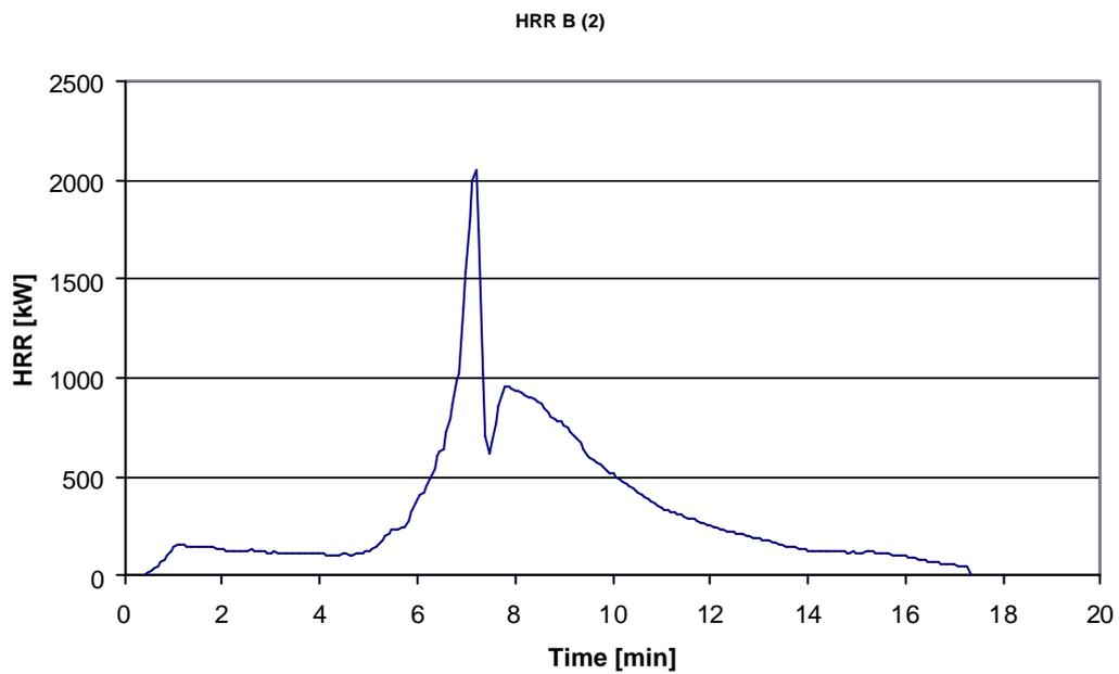
Figure A.4 Heat release rate of product B in ISO 9705
