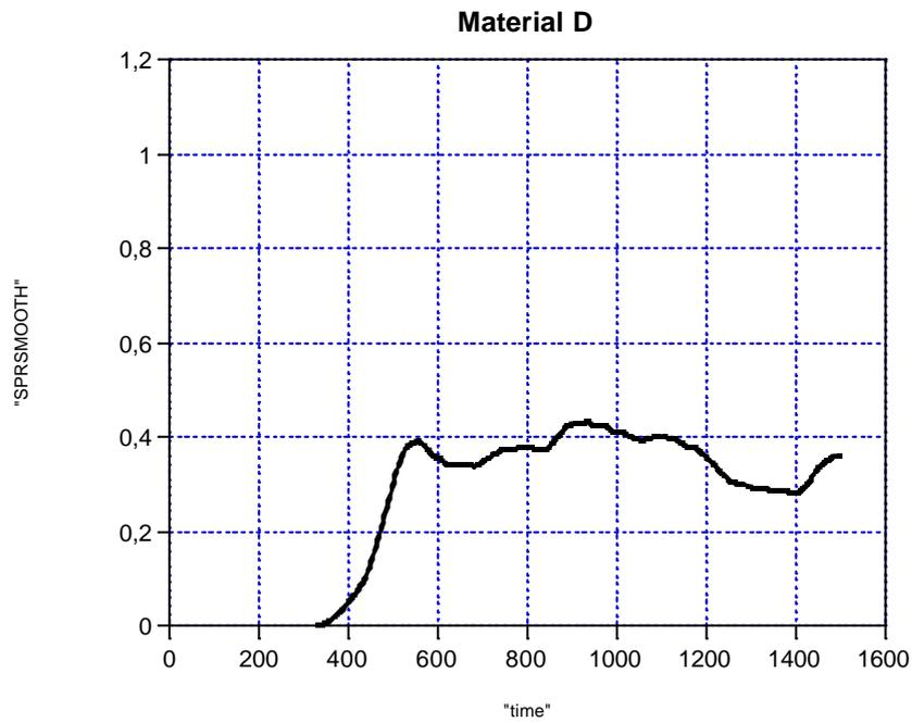
Figure C.8 Smoothed smoke release rate of product D in the SBI test
