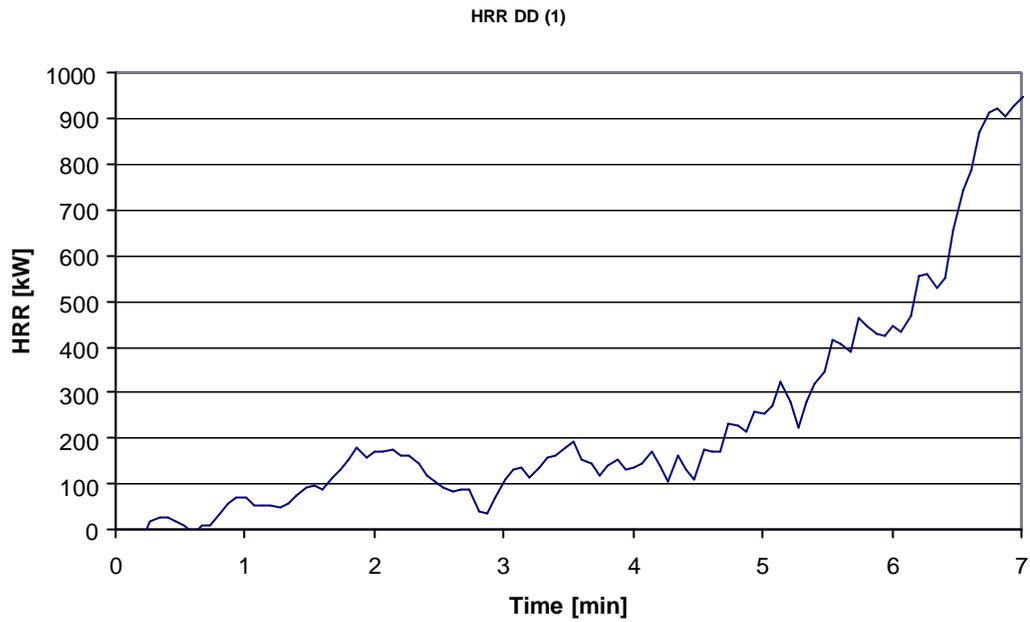
Figure B.9 Detail of heat release rate of product D in free standing set-up
