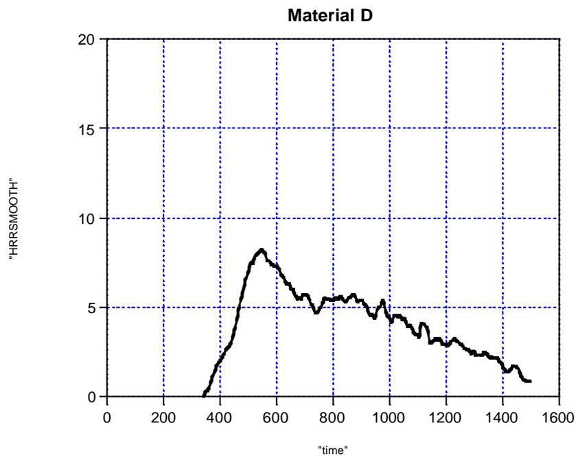
Figure C.4 Smoothed heat release rate of product D in the SBI test
