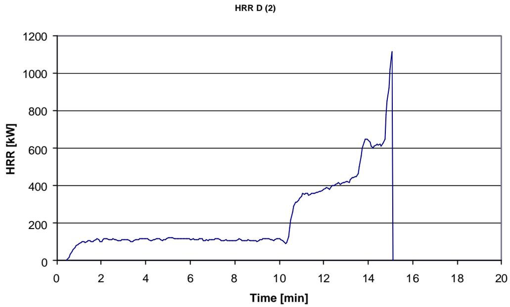
Figure A.9 Heat release rate of product D in ISO 9705
