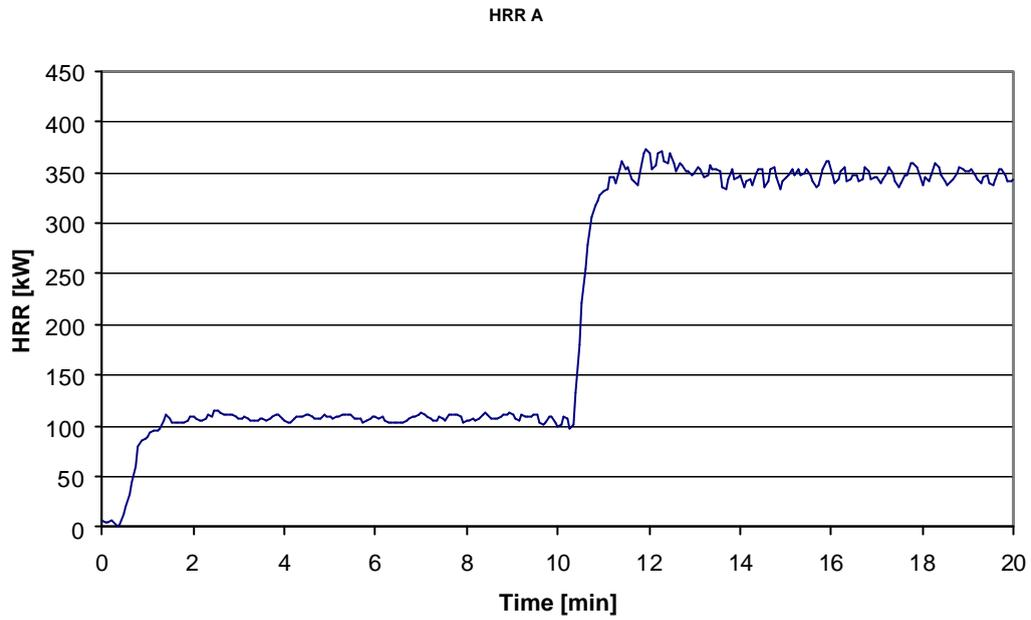
Figure A.1 Heat release rate for product A in ISO 9705
