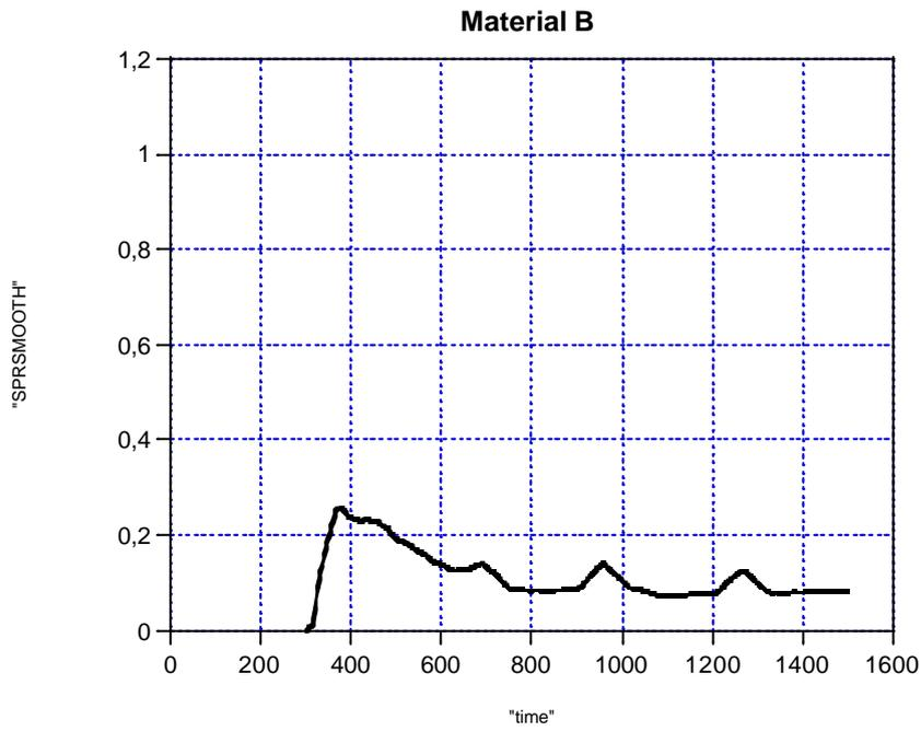
Figure C.6 Smoothed smoke release rate of product B in the SBI test
