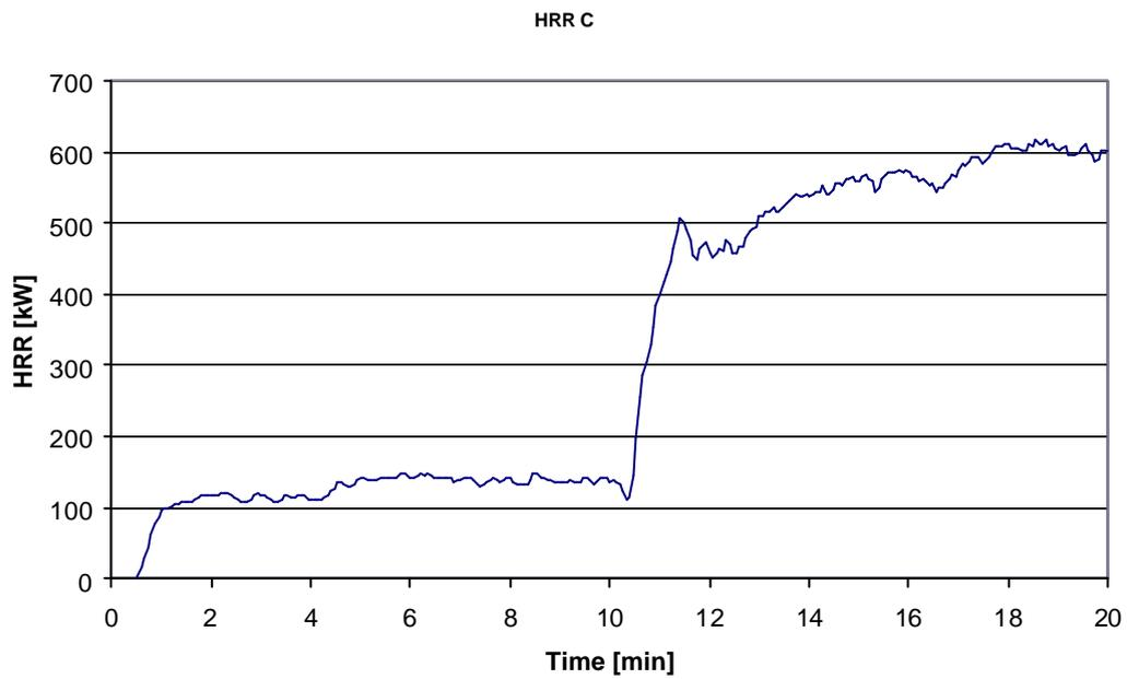
Figure A.6 Heat release rate of product C in ISO 9705
