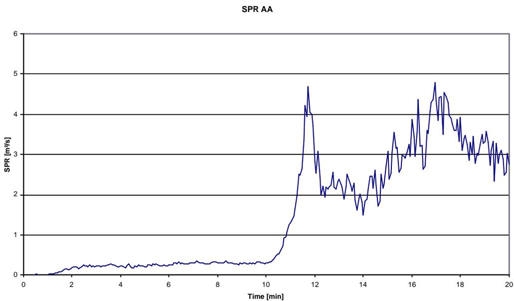
Figure B.2 Smoke production rate of product A in free standing set-up (corrected for soot deposit after 12 minutes)
