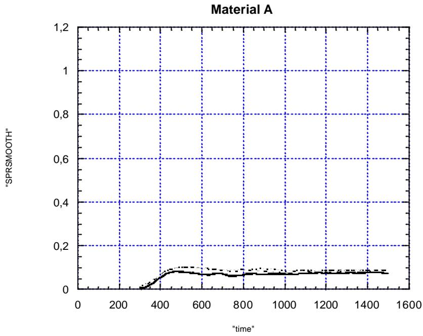
Figure C.5 Smoothed smoke release rate of product A in the SBI test
