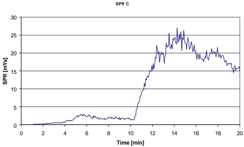
Figure A.7 Smoke production rate of product C in ISO 9705
